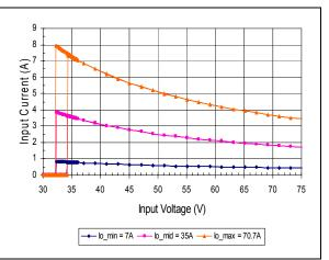
Output Current Limit Characteristics vs. Input Voltage
